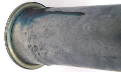
Figure 1 Fuel Staining on the Intake Pipe
