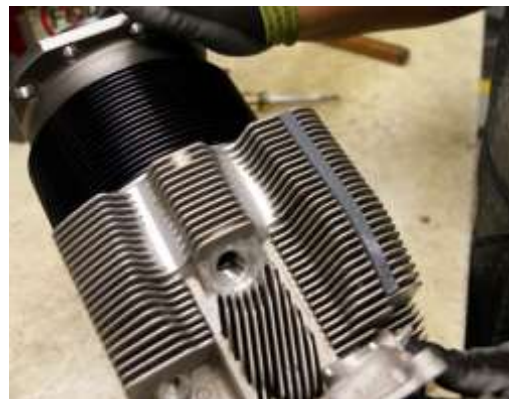
Figure A-5 Fin Stabilizer Installed on Cylinder
