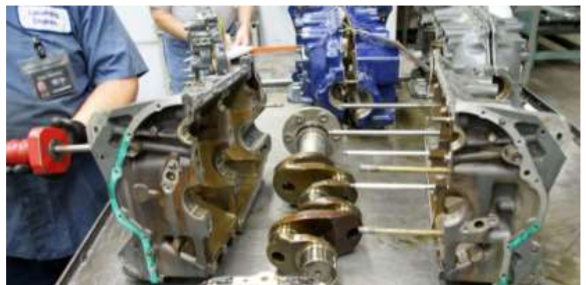
Figure 8 Remove the Crankshaft
