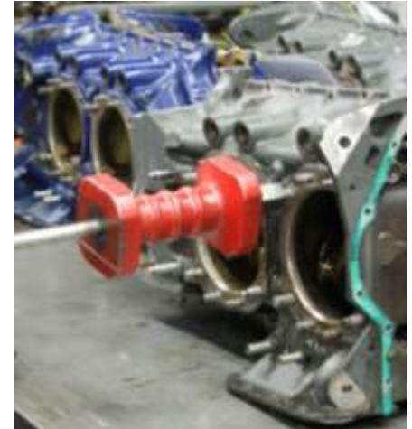
Figure 6 Separate the Crankcase Halves
