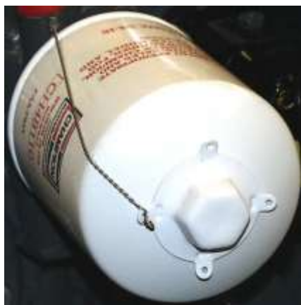
Figure 3 Safety Wire on Oil Filter
