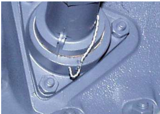
Figure 2 Safety Wire on the Oil Level Gage
