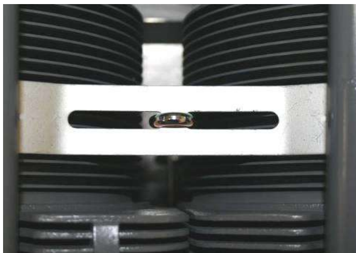
Figure 39 Intercylinder Baffle Installed on Three Fins
