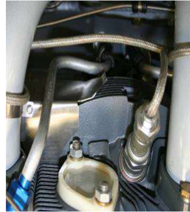
Figure 41 Loose Fit of Intercylinder Baffle
