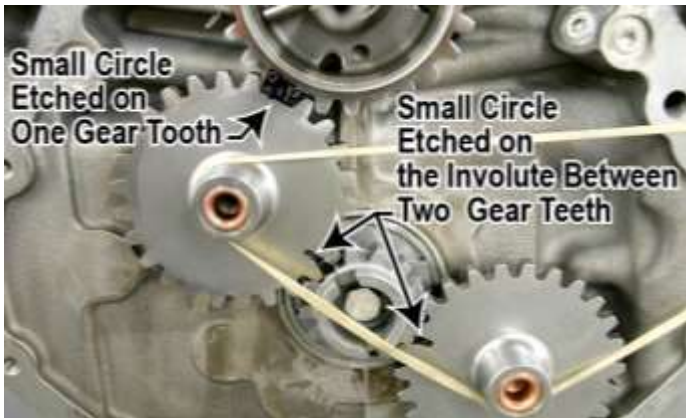
Figure 88 Left Crankshaft Idler Gear
