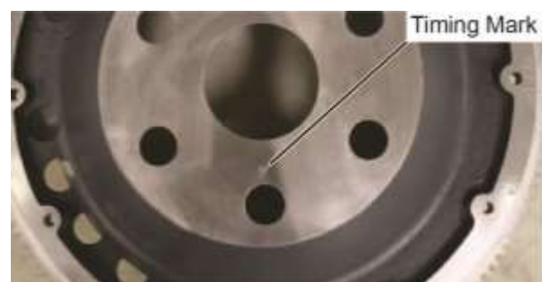
Figure 10 Timing Mark on the Starter Ring Gear
