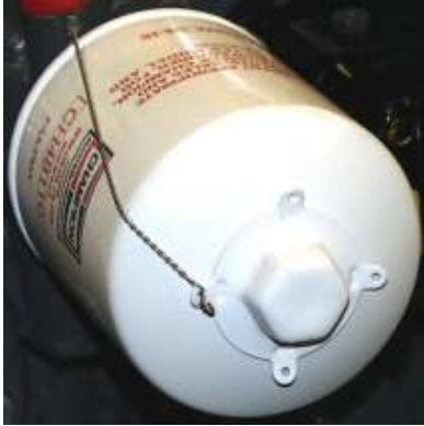
Figure A-10 Safety Wire on Oil Filter
