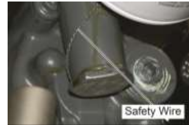
Figure A-13 Safety Wire on the Thermostatic Oil Cooler Bypass Valve
