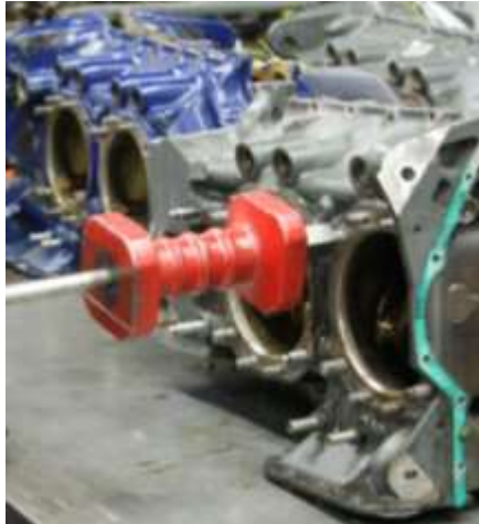
Figure 4 Attach the Slide-Hammer to a Base Stud
