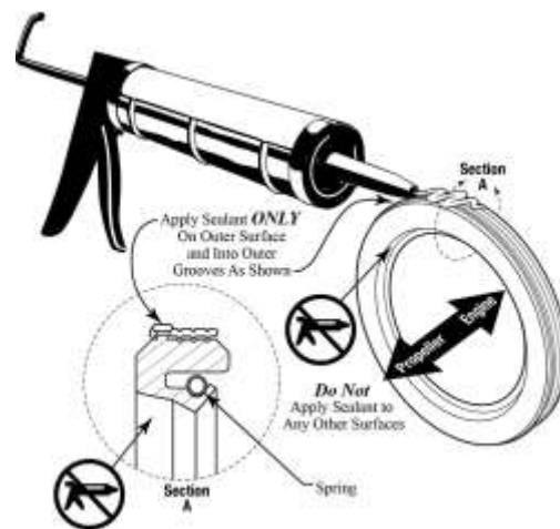
Figure 82 Apply the Sealant Only on the Outer Surface of the Oil Seal
