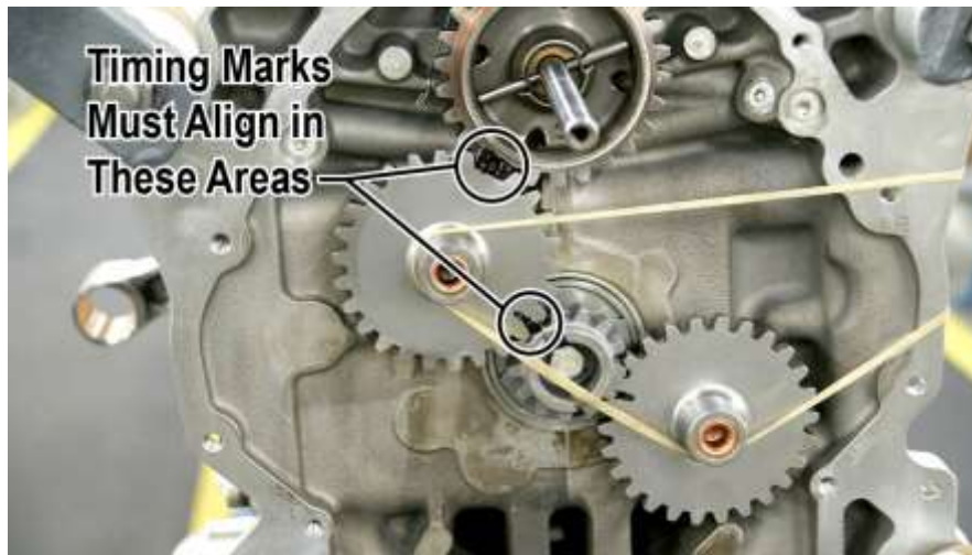
Figure 92 Rubber Band to Hold Crankshaft Idler Gears
