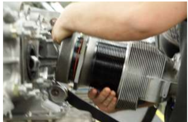
Figure 27 Install the Cylinder
