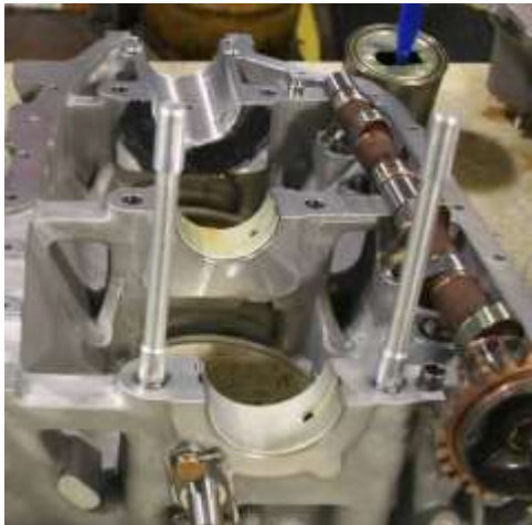
Figure 65 Thrust Bearing Surfaces of Each Crankcase Half
