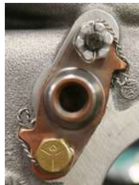
Figure 55 Safety Wiring the Crankshaft Idler Gear Shaft
