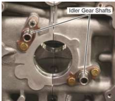
Figure 54 Shaft Installation in the Crankcase for Left and Right Crankshaft Idler Gears
