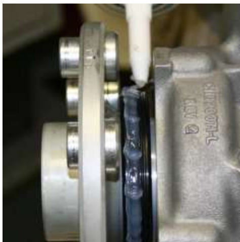
Figure 81 Apply the Sealant to the Oil Seal
