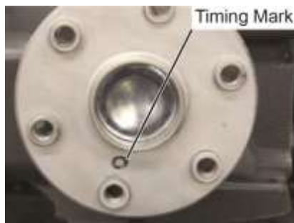
Figure 9 Timing Mark on the Crankshaft Flange
