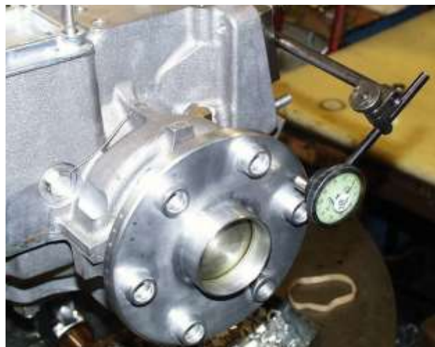
Figure 80 Crankshaft End Play Check
