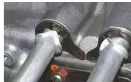
Figure 33 Correctly Aligned Shroud Tube Springs
