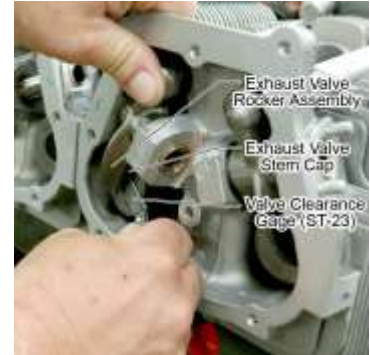
Figure 36 Measuring Dry Tappet Clearance
