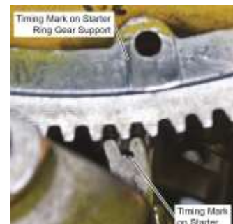
Figure 2 Timing Marks on the Front Side of the Starter Ring Gear Support Assembly Aligned with the Timing Mark on the Starter
