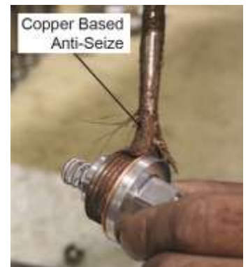
Figure 6 Apply Copper Based Anti-Seize to Threads
