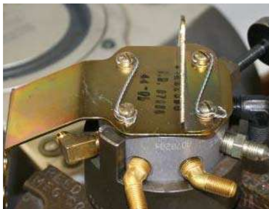
Figure 11 Safety Wire the Screws
