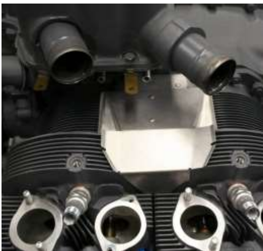
Figure 38 Placement of Intercylinder Baffle on Down Exhaust Engines
