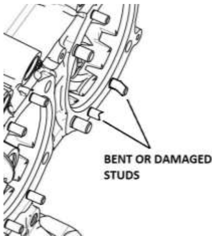
Figure A-1 Damaged Studs
