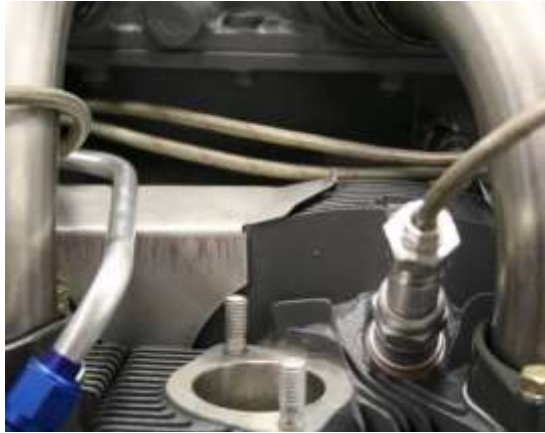
Figure 40 Correct Tight Fit of Intercylinder Baffle
