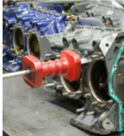
Figure 5 Strike the Slide Part of the Tool Against the Back of the Tool
