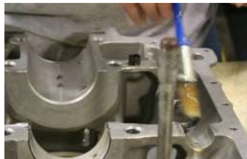
Figure 76 Lubricant Application to Camshaft Bearing Saddle in Crankcase Half
