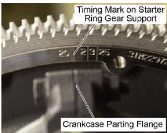
Figure 8 Timing Marks on the Crankcase Side of the Starter Ring Gear Support Aligned with the Crankcase Parting Flange
