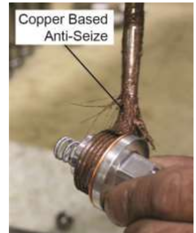
Figure 6 Apply Copper Based Anti-Seize to Threads
