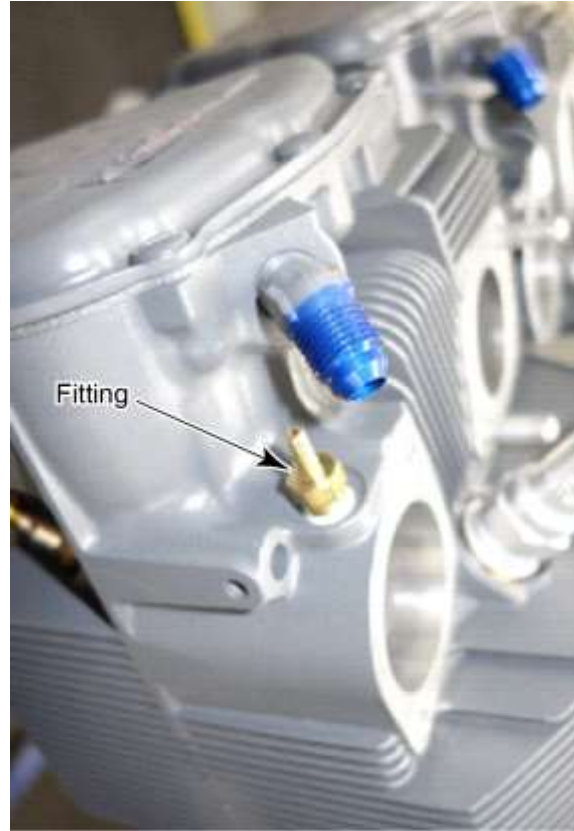
Figure A-9 Fitting Installed in the Cylinder
