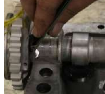
Figure 74 Camshaft End Play Clearance Check
