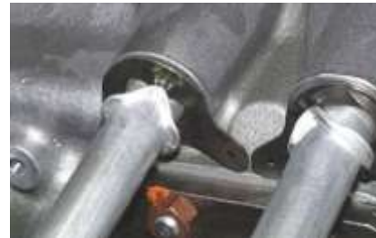
Figure 34 Correctly Aligned Shroud Tube Springs
