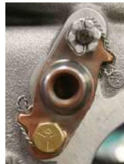
Figure 60 Safety Wire on the Crankshaft Idler Gear Shaft
