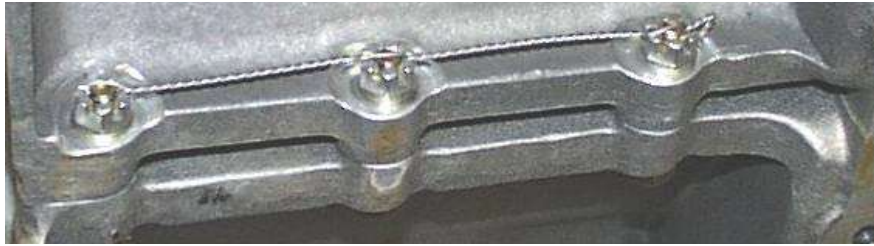
Figure 91 Safety Wire Nuts in Crankcase Oil Sump
