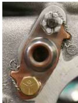
Figure 17 Safety Wire on the Idler Gear Shaft
