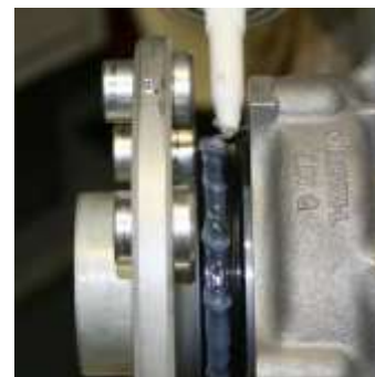
Figure 92 Apply the Sealant to the Oil Seal
