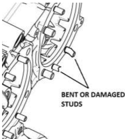
Figure A-1 Damaged Studs
