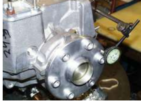
Figure 98 Crankshaft Endplay Check
