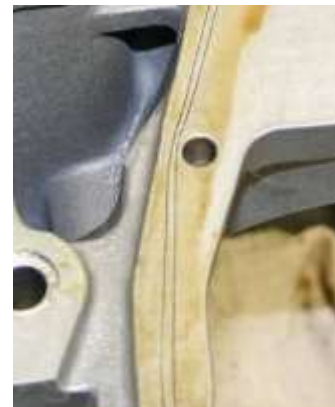
Figure 83 Placement of Silk Threads Along Inside Edge of Crankcase Flange
