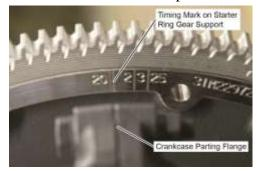
Figure 1 Timing Marks on the Crankcase Side of the Starter Ring Gear Support Aligned with the Crankcase Parting Flange
