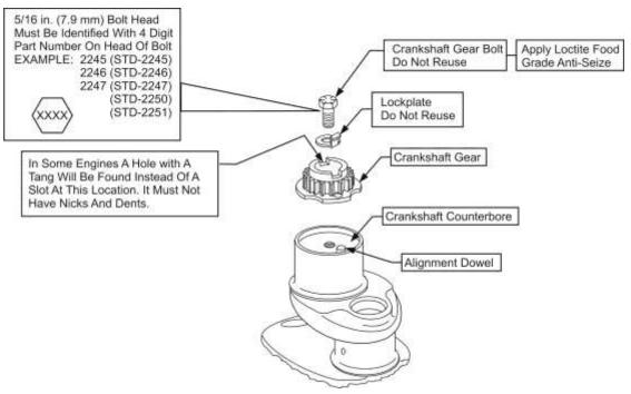
Figure 27 Crankshaft Gear Bolt and Lockplate
