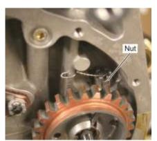
Figure 89 **Nut on Stud at Rear Camshaft Bearing**
