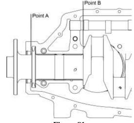
Figure 81 Clearance Between Crankshaft and Crankcase
