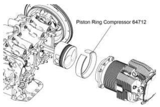
Figure 26 Piston Ring Compressor (64712)
