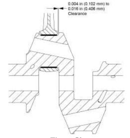
Figure 52 Connecting Rod Clearance
