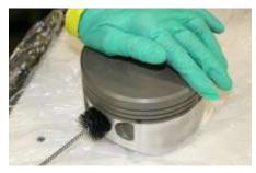
Figure 1 Cleaning the Piston Pin Bore with a Soft Bristle Non-Metallic Brush
