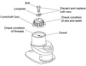
Figure 20 **Crankshaft Gear and Associate Parts**
