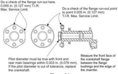
Figure 26 **Crankshaft Flange Run-Out and Pilot Diameter**
