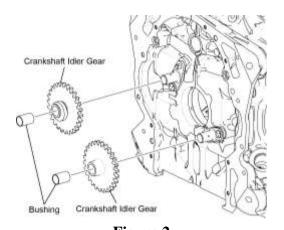
Figure 2 Crankshaft Idler Gears
