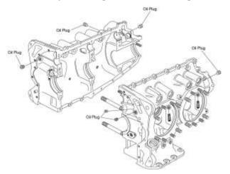
Figure 16 Oil Plugs in the Crankcase
