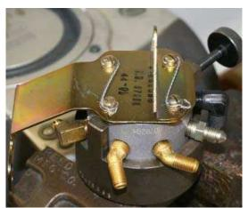
Figure 11 Safety Wire the Screws
