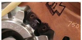
Figure 94 Correct Alignment Between the Crankshaft Gear and the Left Crankshaft Idler Gear
