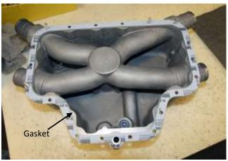
Figure 13 Oil Sump Gasket
