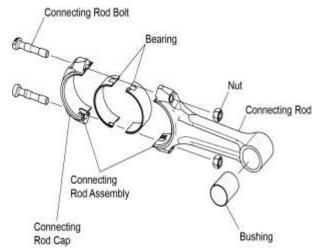
Figure 1 Connecting Rod Parts
