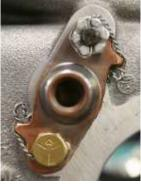
Figure 17 Safety Wire on the Crankshaft Idler Gear Shaft
