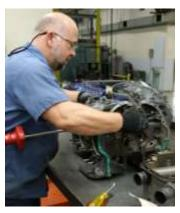
Figure 6 Separate the Crankcase Halves
