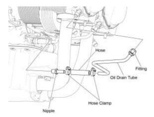
Figure 37 Oil Drain Tube
