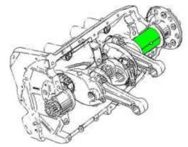
Figure 80 Crankshaft Installed in Crankcase Half
