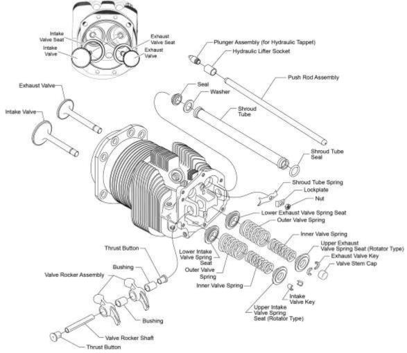
Figure 15 LIO-360-B1G6 Engine Valve Components
