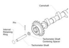
Figure 33 **Camshaft with Integral Gears**
