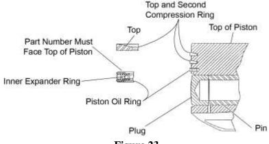
Figure 23 **Piston Ring Positions**
