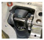
Figure 68 Propeller Governor Idler Gear Shaft
