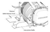
Figure 14 Intercylinder Baffles
