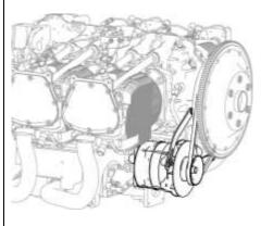
Figure 37 Alternator Bracket, Alternator, and Alternator Belt
