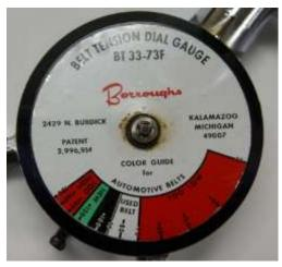
Figure 3 Indicator on the Belt Tension Dial Gage (ST-131)
