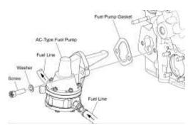
Figure 12 AC-Type Fuel Pump
