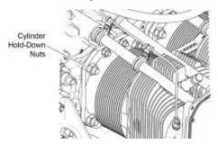
Figure 16 Cylinder Base Hold-Down Nuts
