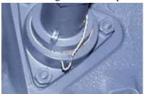
Figure 2 Safety Wire on the Oil Level Gage
