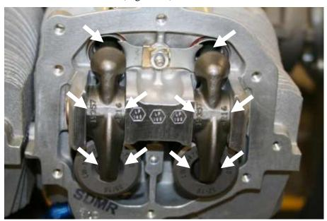
Figure 36 Valve Rocker Lubrication
