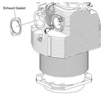
Figure 1 Exhaust Gasket
