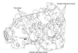
Figure 25B Crankcase Thru-Studs and Cylinder Hold-Down Studs
