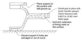
Figure 11 Starter Ring Gear Support
