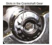
Figure 5 Slots in the Crankshaft Gear
