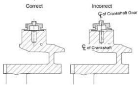
Figure 44 Crankshaft Gear Position
