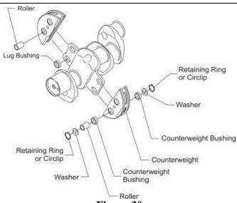
Figure 30 Crankshaft Counterweight, Rollers, and Bushings
