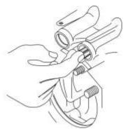
Figure 10 **Removing Push Rod Socket**
