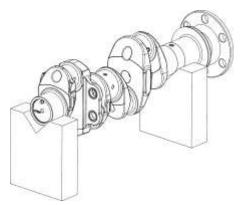
Figure 9 Crankshaft in V-Block-Type Fixture
