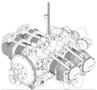
Figure 1 **Lifting Strap**
