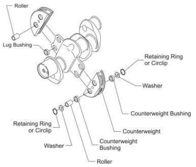
Figure 22 Counterweight, Rollers, Counterweight Bushings, and Lug Bushings (Crankshaft Dynamic Counterweight Bushings)
