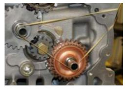
Figure 97 Rubber Band to Hold Crankshaft Idler Gears
