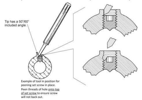
Figure 71 Center Punch (Peening Tool) for Set Screw
