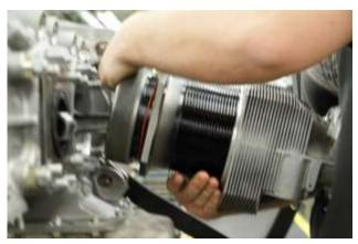
Figure 27 **Install the Cylinder**
