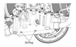
Figure 15 Oil Plugs in the Oil Sump
