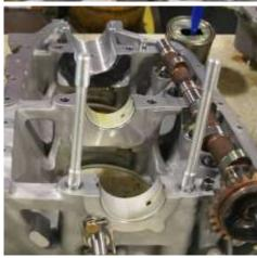
Figure 76 **Thrust Bearing Surfaces** of Each Crankcase Half
