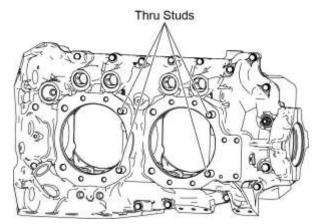
Figure 3 Crankcase Assembly
