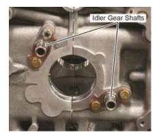
Figure 18 Crankshaft Idler Gear Shafts
