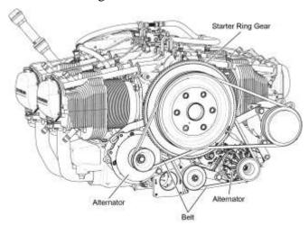
Figure 1 Alternator and Alternator Belt
