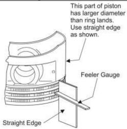
Figure 22 Checking Piston Ring Side Clearance
