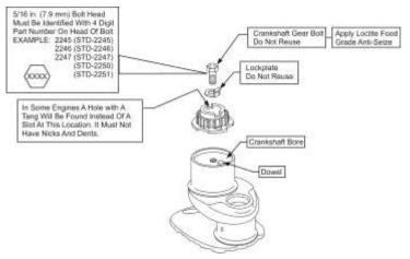
Figure 43 Crankshaft Gear Bolt and Lockplate
