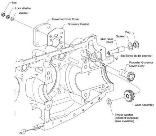
Figure 13 Propeller Governor Drive
