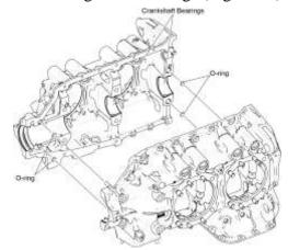
Figure 66 Center and Rear Main Bearings, Bolts, and O-Rings
