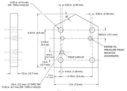
Figure 99 ST-483 Test Plate
