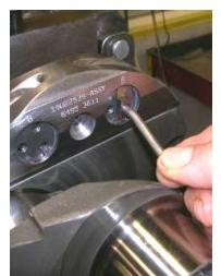
Figure 55 Circlip Check Gage P/N 64892-2
