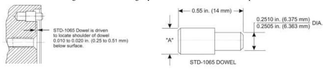
Figure 31 Section Through Counterbore End of Crankshaft Showing Driven Height of Dowel
