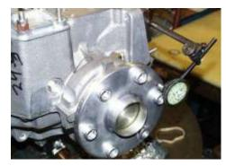
Figure 98 Crankshaft End Play Check
