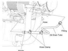
Figure 12 Oil Drain Tube
