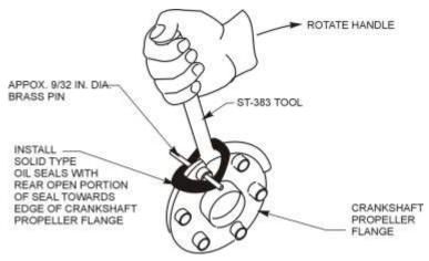
Figure 49 Crankshaft Propeller Flange Showing the Installation of the Solid-Ring Oil Seal
