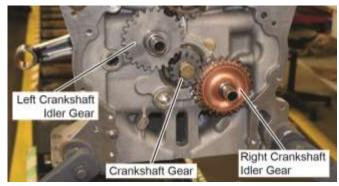
Figure 96 Crankshaft Idler Gears Installed
