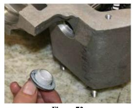
Figure 72 Idler Gear Shaft Plug
