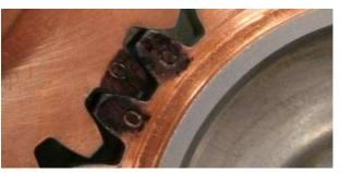
Figure 95 Correct Alignment Between the Camshaft Gear and the Right Crankshaft Idler Gear
