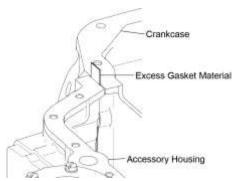
Figure 11 Remove Excess Accessory Housing Gasket to Make It Flush with the Oil Sump Flange
