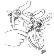
Figure 11 **Removing Hydraulic Tappet Plunger Assembly**
