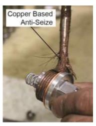
Figure 6 **Apply Copper Based Anti-Seize to Threads**
