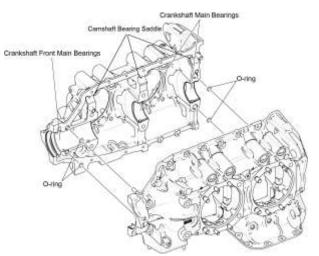
Figure 12 **Main Bearings and O-Rings**
