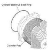
Figure 17 Cylinder Base Oil Ring and Cylinder Fins
