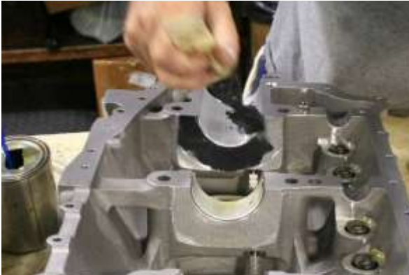
Figure 85 Thrust Bearing Surfaces and Main Bearings of Each Crankcase Half
