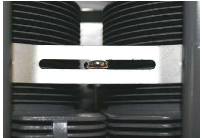
Figure 41 Intercylinder Baffle Installed on Three Fins
