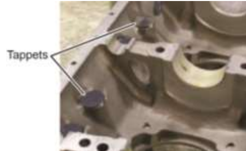
| Figure 73 Installed Tappets
