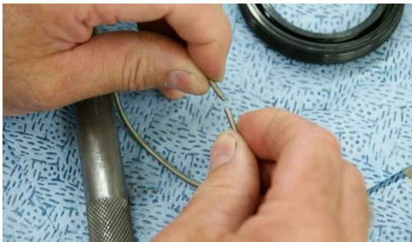
Figure 57 Separating the Spring Threaded Ends
