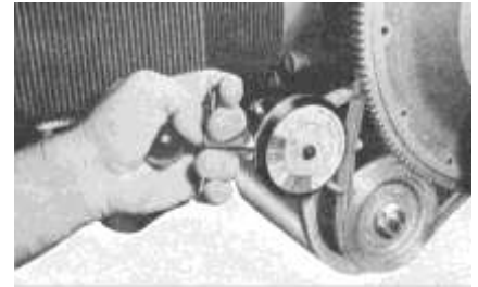
Figure 2 Belt Tension Gage - ST-131
