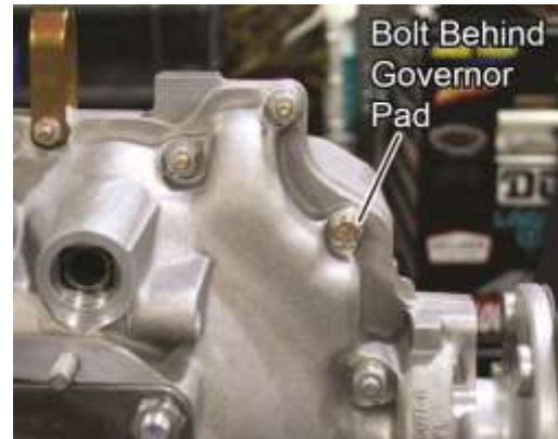
Figure 99 Bolt Behind Governor Pad
