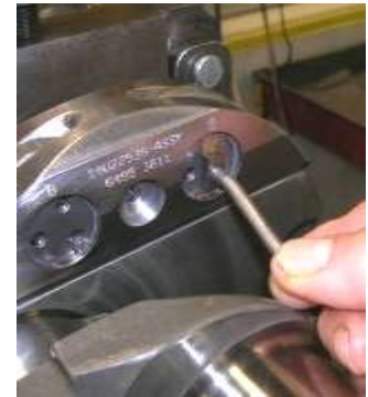
Figure 68 Insertion of Circlip Check Gage
