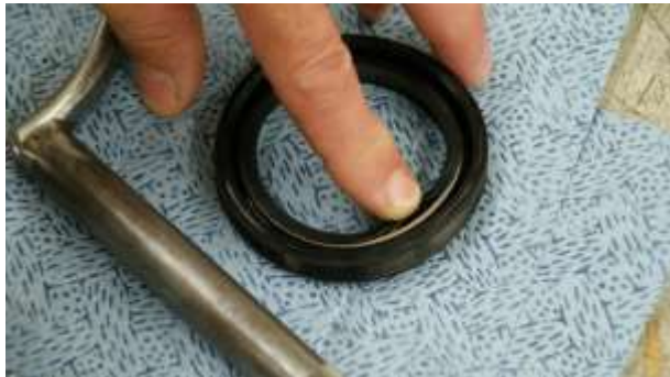
Figure 55 Locating the Internal Spring
