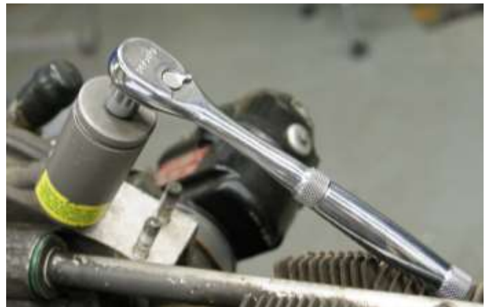
Figure A-2 Stud Removal Tool
