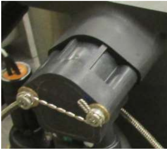
Figure 38 Safety Wire on the Throttle Position Sensor
