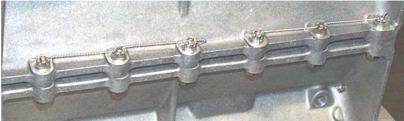
Figure 100 Safety Wire on the Nuts in the Crankcase Oil Sump
