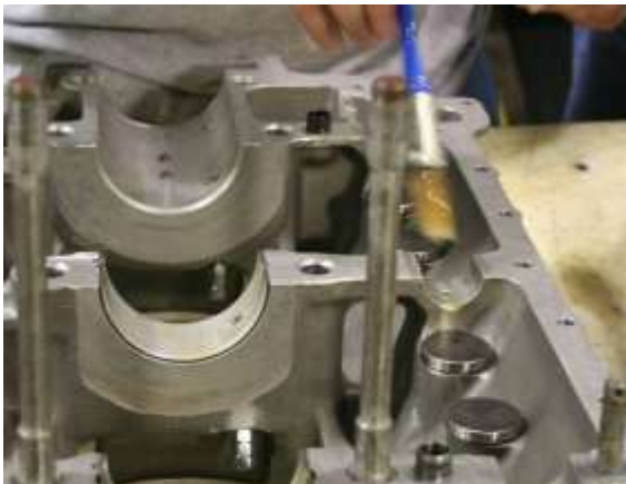
Figure 86 Lubricant the Camshaft Bearing Saddle in Each Crankcase Half
