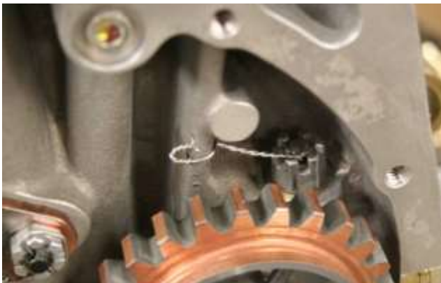
Figure 98 Nut on Stud at Rear Camshaft Bearing
