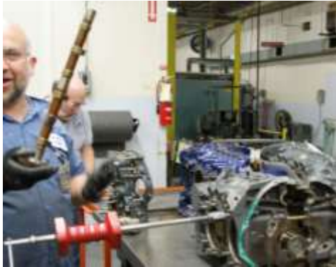
Figure 8 Remove the Camshaft
