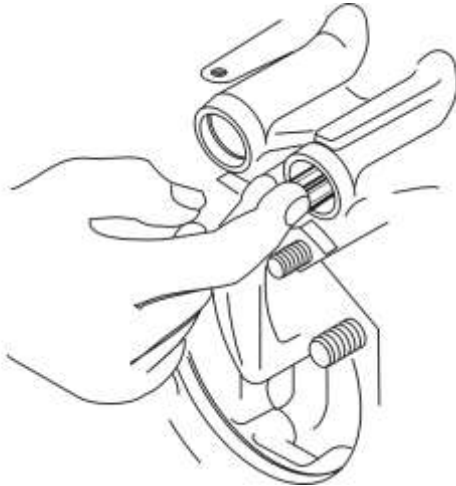
Figure 11 Removing Push Rod Socket
