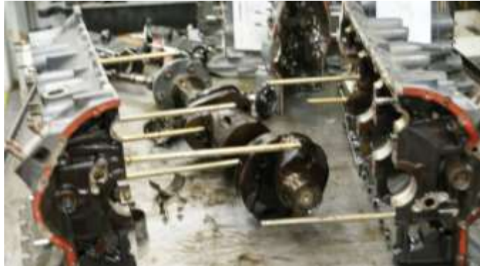
Figure 9 Remove the Crankshaft
