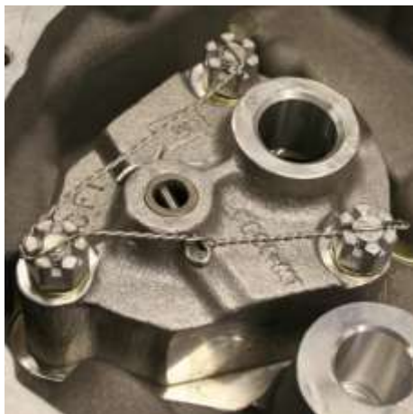
Figure 3 Safety Wire on the Oil Pump
