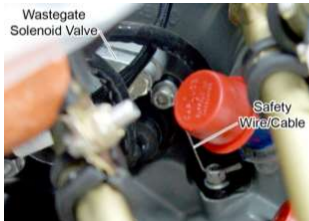
Figure 9 Safety Wire/Cable on Wastegate Solenoid Valve Bolt
