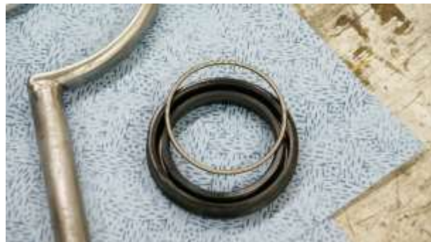
Figure 56 Internal Spring Removed
