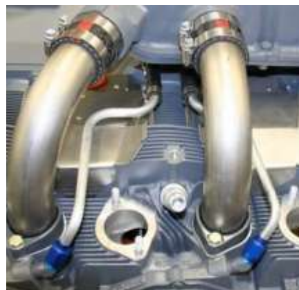
Figure 45 Oil Drain Tubes, Clamps, and Fittings
