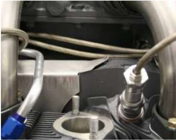
Figure 42 Correct Tight Fit of Intercylinder Baffle
