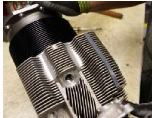
Figure A-5 Fin Stabilizer Installed on Cylinder
