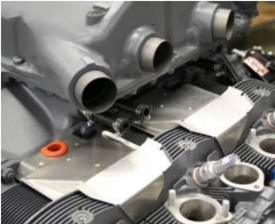
Figure 40 Placement of Intercylinder Baffle on Down Exhaust Engines
