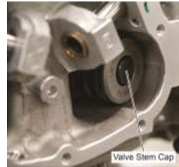
Figure 10 Exhaust Valve Stem Cap
