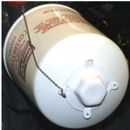
Figure 4 Safety Wire on Oil Filter
