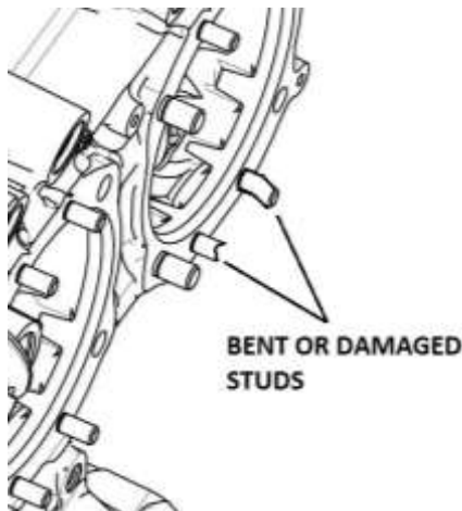
Figure A-1 Damaged Studs
