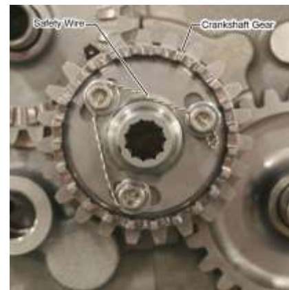
Figure 3 Safety Wire on the Fuel Pump Shaft Drive Screws
