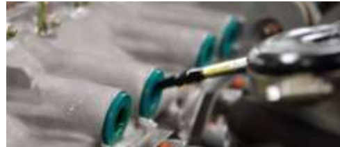
Figure 32 Shroud Tube Oil Seals in Crankcase
