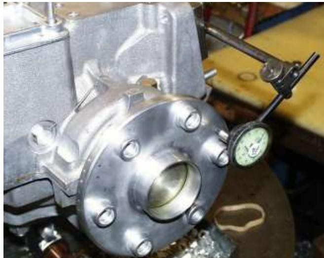
Figure 101 Crankshaft End Play Check
