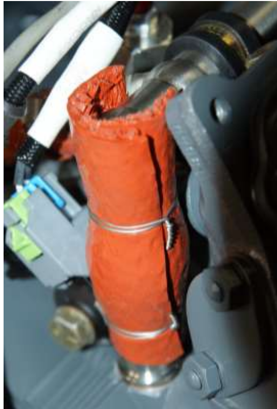
Figure 11 Installed Fire Sleeve P/N 01M29869
