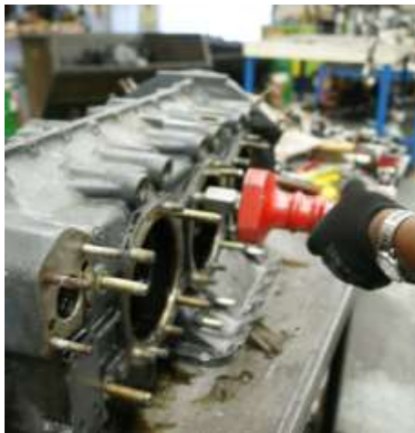
Figure 5 Attach the Slide-Hammer to a Base Stud
