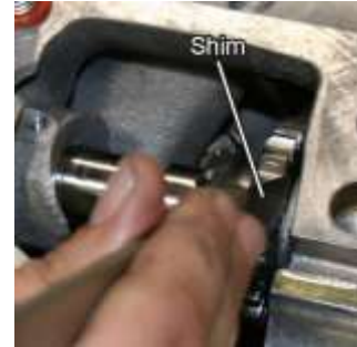
Figure 78 Shim Between Spacer and Crankcase – Backlash Check
