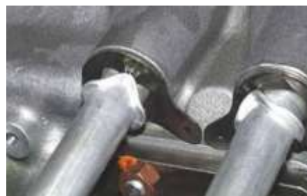
Figure 35 Correctly Aligned Shroud Tube Springs
