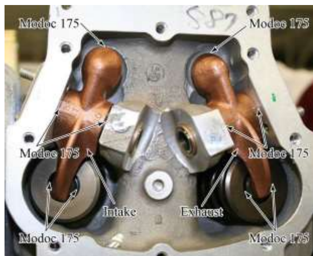
Figure 39 Valve Rocker Lubrication
