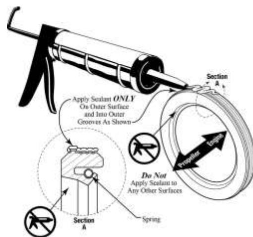
Figure 105 Apply the Sealant Only on the Outer Surface of the Oil Seal
