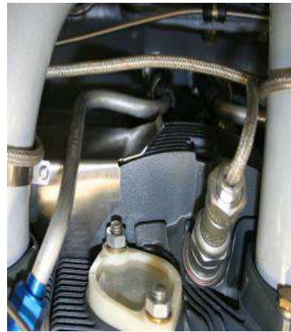
Figure 43 Loose Fit of Intercylinder Baffle
