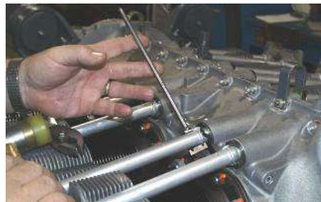
Figure 34 Shroud Tube Wrench ST-142
