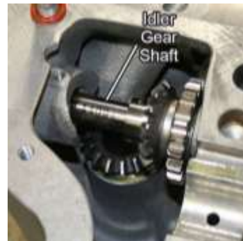
Figure 77 Propeller Governor Idler Gear Shaft
