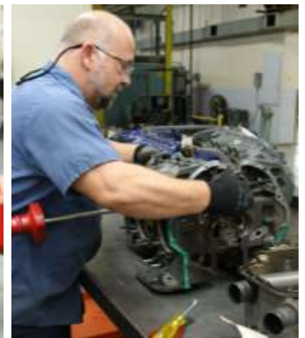
Figure 7 Separate the Crankcase Halves
