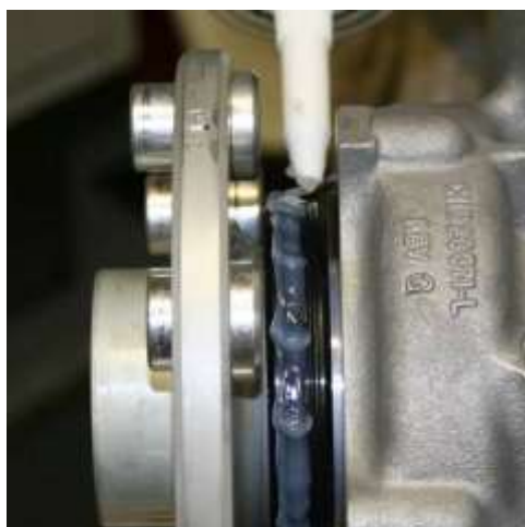
Figure 104 Apply the Sealant to the Oil Seal
