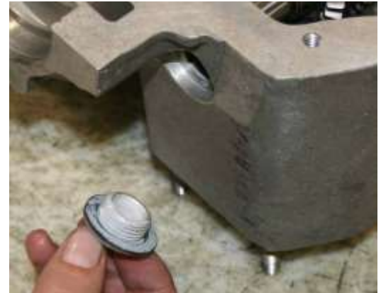
Figure 81 Idler Gear Shaft Plug
