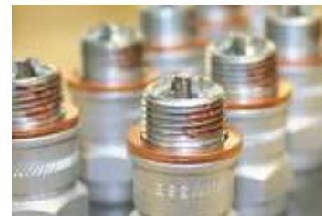
Figure 6 Copper-Based Anti-Seize Applied to Spark Plug Threads
