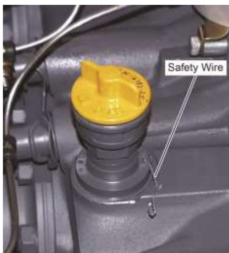
Figure 2 Safety Wire on the Oil Filler Extension
