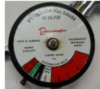
Figure 3 Indicator on the Belt Tension Gage (ST-131)
