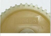
Figure 3. Affected K3008 Distributor Figure 4. K3008 Distributor Gear Gear With Copper Electrode Marked 510406 (Backside)
