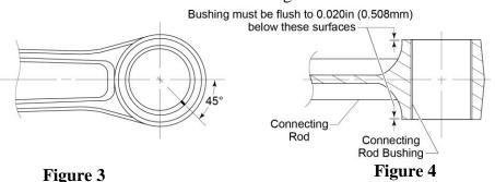
Bushing Installed in the Connecting Rod
