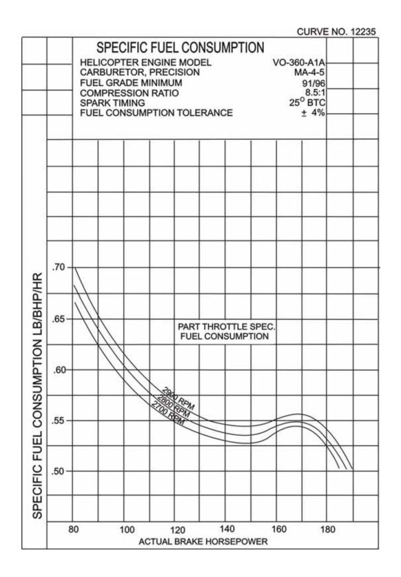
Figure 3-1. Fuel Consumption Curve - VO-360-A1A
