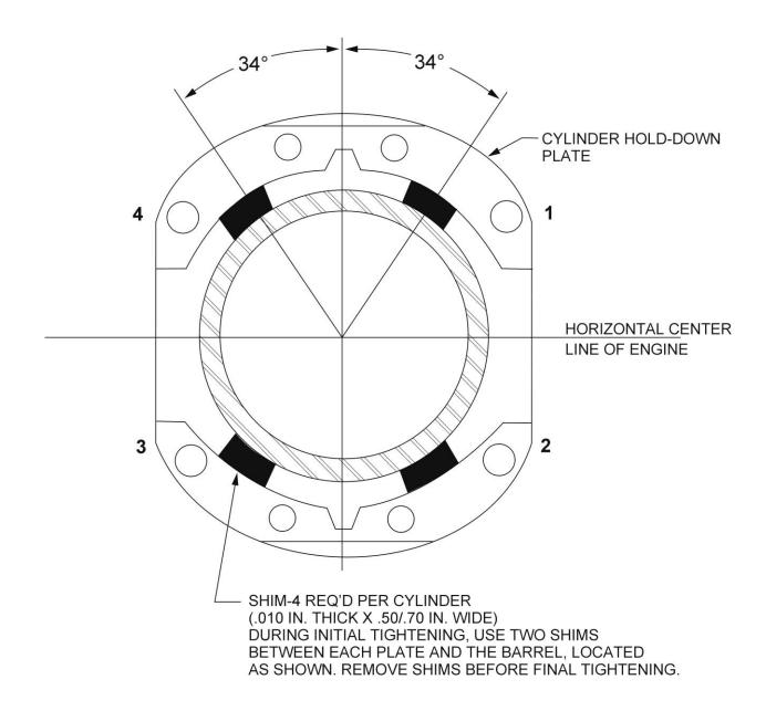
Figure 5-2. Location of Shims Between Cylinder Barrel and Hold Down Plates and Sequence of Tightening Cylinder Base Hold Down Nuts
