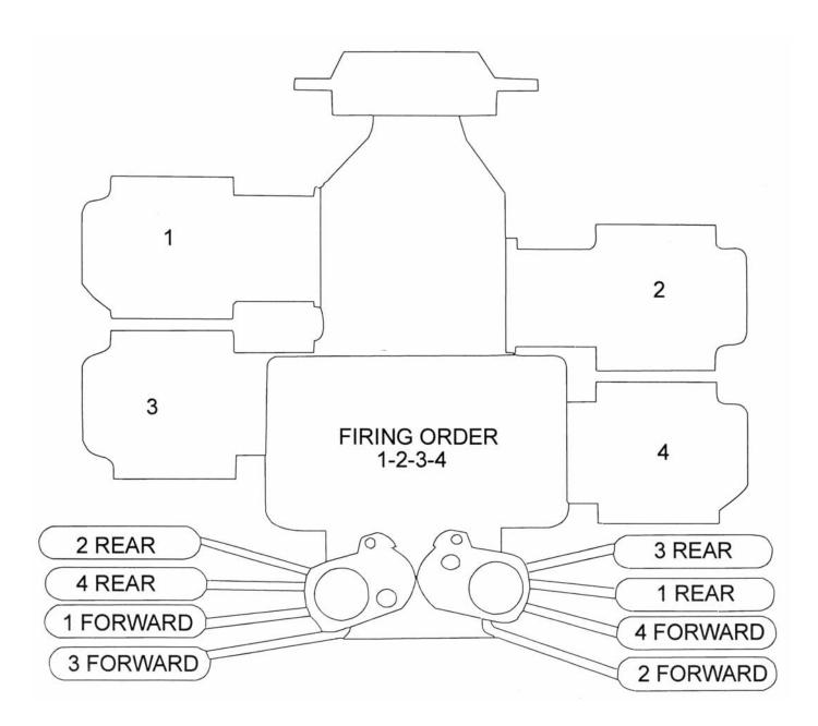
Figure 5-1. Ignition Wiring Diagram
