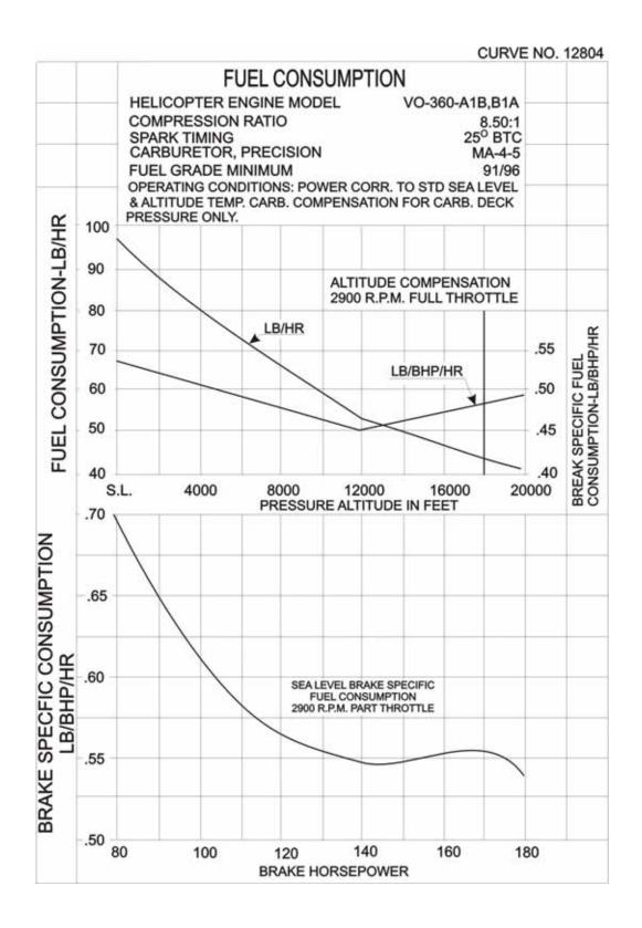
Figure 3-3. Fuel Consumption Curve - VO-360-A1B, -B1A
