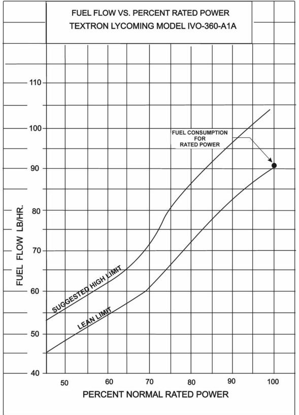
Figure 3-6. Fuel Flow vs Percent Rated Power - IVO-360-A1A
