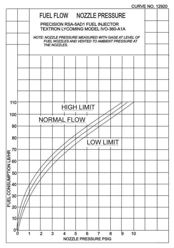
Figure 3-5. Fuel Flow vs Nozzle Pressure – IVO-360-A1A
