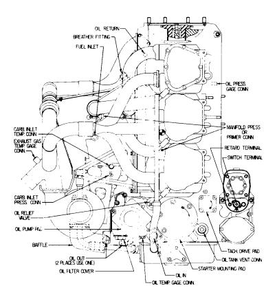
Figure 7-6. Installation Drawing - Right Side - TVO-435-D Series
