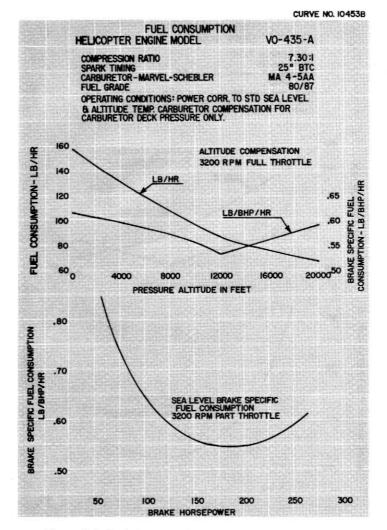
Figure 3-1. Fuel Consumption Curve - VO-435-A Series
