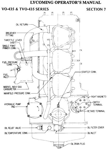
Figure 7-3. Installation Drawing - Right Side - VO-435-B Series
