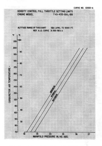
Figure 5-6. Density Control Full Throttle Setting Limits TVO-435-B1A, -B1B
