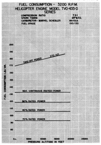
Figure 3-5. Fuel Consumption Curve - TVO-435-D Series
