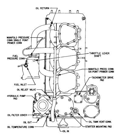
Figure 7-1. Installation Drawing - Right Side - VO-435-A Series
