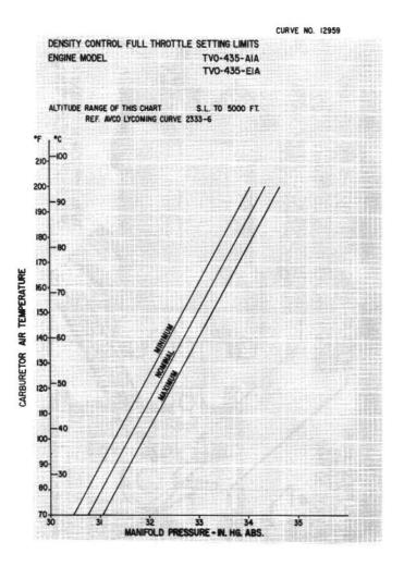
Figure 5-5. Density Control Full Throttle Setting Limits TVO-435-A1A, -E1A
