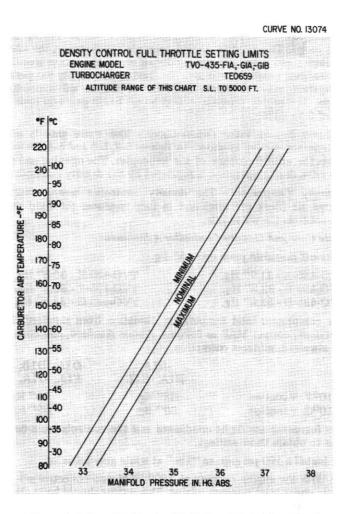
Figure 5-8. Density Control Full Throttle Setting Limits TVO-435-F1A, -G1A, -G1B
