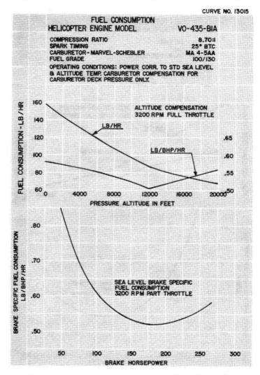
Figure 3-2. Fuel Consumption Curve - VO-435-B Series
