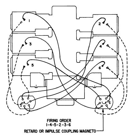
Figure 5-1. Ignition Wiring Diagram
